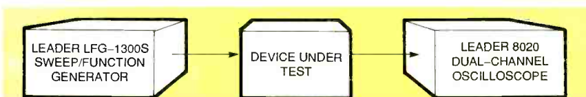
Fig. 2. Our benchmark test bench is built around a Leader Model LFG-1300S sweep/function generator and a Leader Model 8020 dual-channel oscilloscope.
